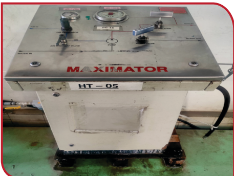
TESTING PUMP 3000 BAR CAPACITY
